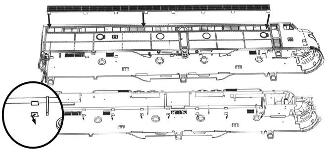
Now insert the tabs on the new grilles into the slots in the body shell, then bend them over on the inside using a screwdriver.
