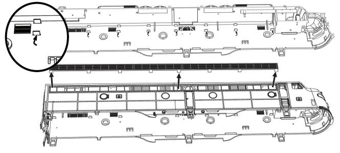
The factory-installed grilles are held in place by several tabs which are bent over inside the shell. To remove them, simply bend the tabs up straight and then push them out. Carefully inserting a hobby knife blade between the body and grille on the outside, then prying up may help.
