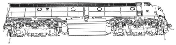
To start, remove the body from the chassis by removing the coupler box screws then sliding the coupler boxes out. Spread the body side slightly to disengage the small clips inside and pull up.
